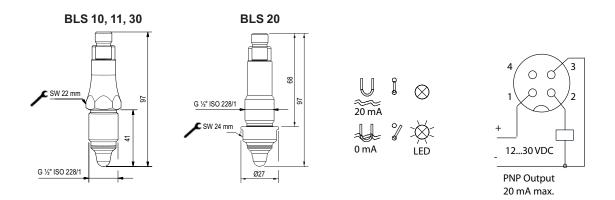
The tip of the sensor is made of PEEK plastic. The sensor works on the principle of frequencysweep technology. The sensor output can be switched from digital to pulse width modulation (PWM). The sensor recognizes different media and can therefore be used for media separation. The analysis of the PWM signal must be done in the connected control unit (PLC).
