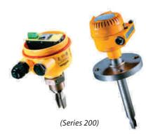
A single point liquid level switch using vibrating Fork wetside, similar to a tuning fork, to detect the presence of a liquid.
