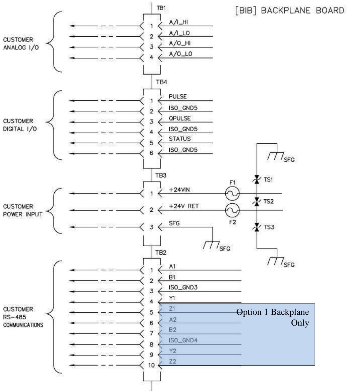
Figure 4.7: User Terminations, Schematic
