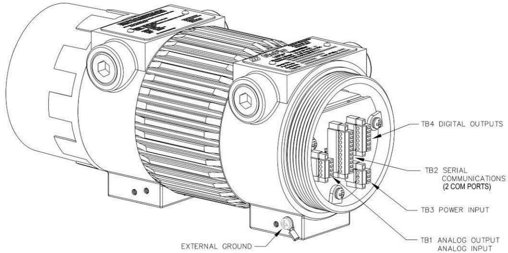
Figure 4.3: User Terminations - Cover Off (Communications Option 1)
