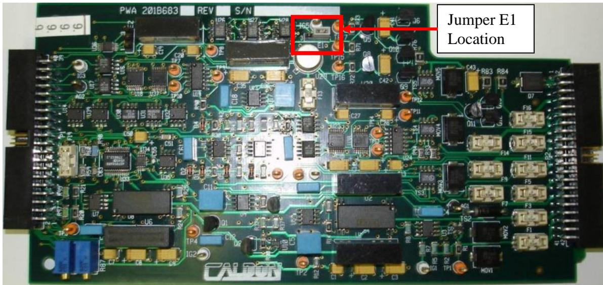
Figure 8.15: Jumper Location to Change Digital Output Voltage
