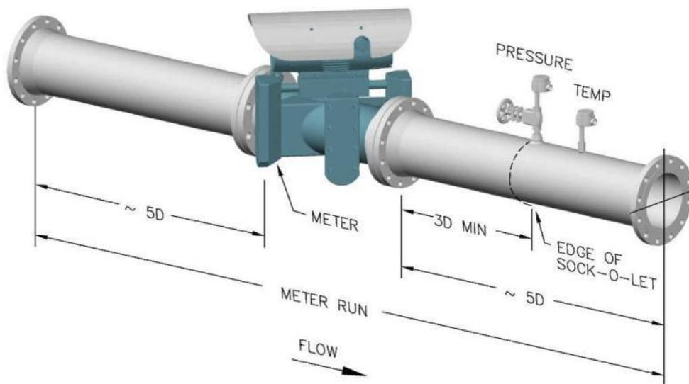
Figure 2.1: 8-Path Meter Best Practice for Installation Hydraulics
