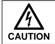
**This symbol indicates actions or procedures which if not performed correctly may lead to personal injury or incorrect function of the instrument or connected equipment.**
