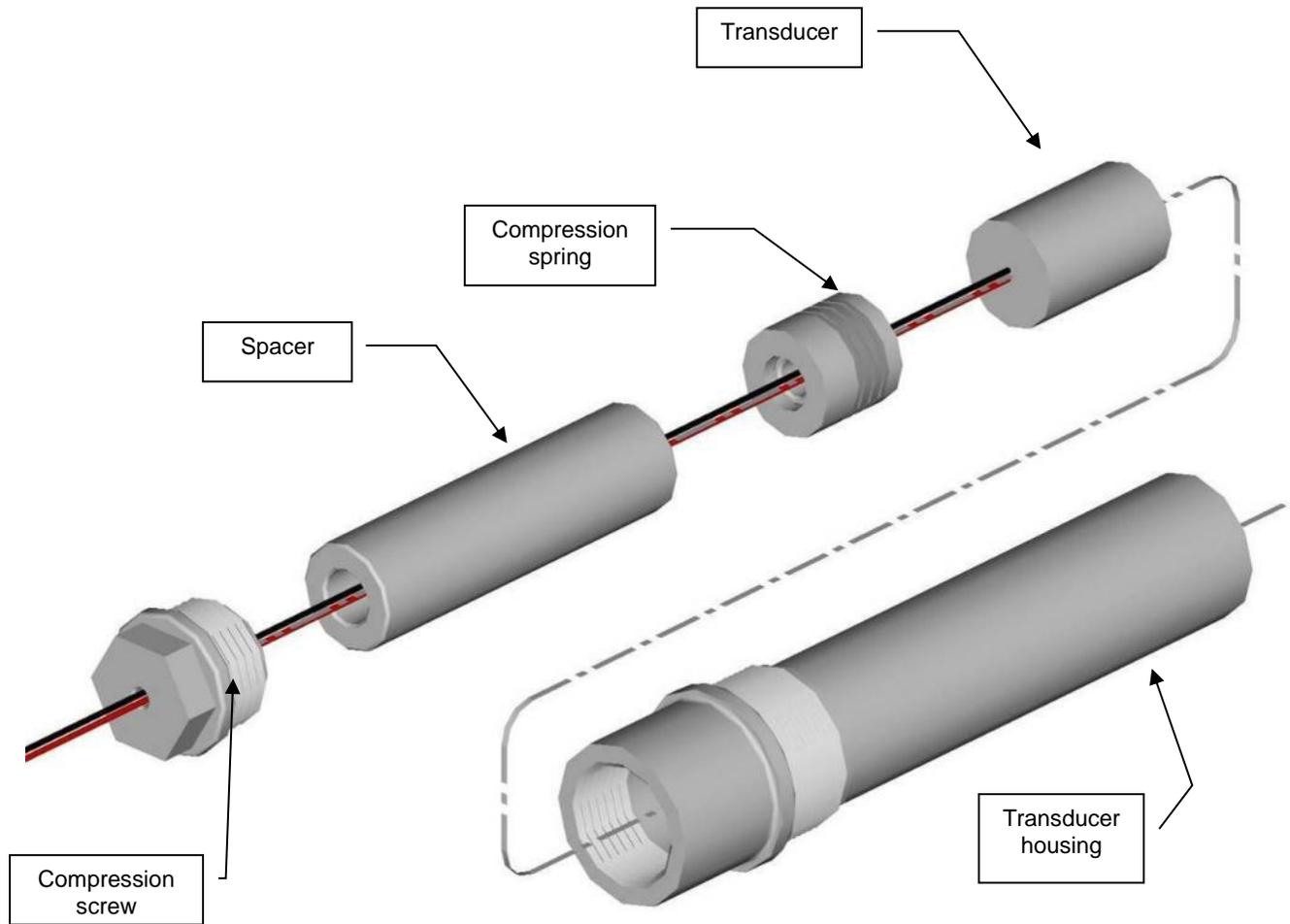
Figure 8.14: Transducer Assembly Construction (half inch housing shown – for the 1 inch housing – the spring and spacer order is reversed).
