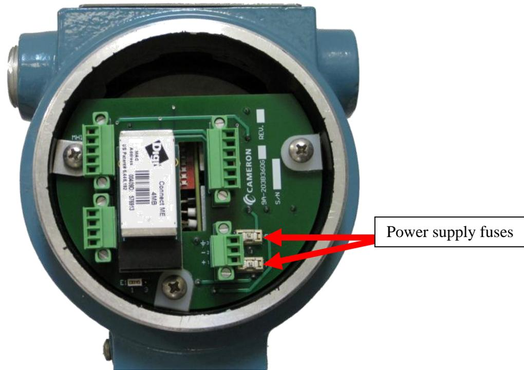
Figure 8.10: Backplane Interface Board (BIB) Fuse Location
