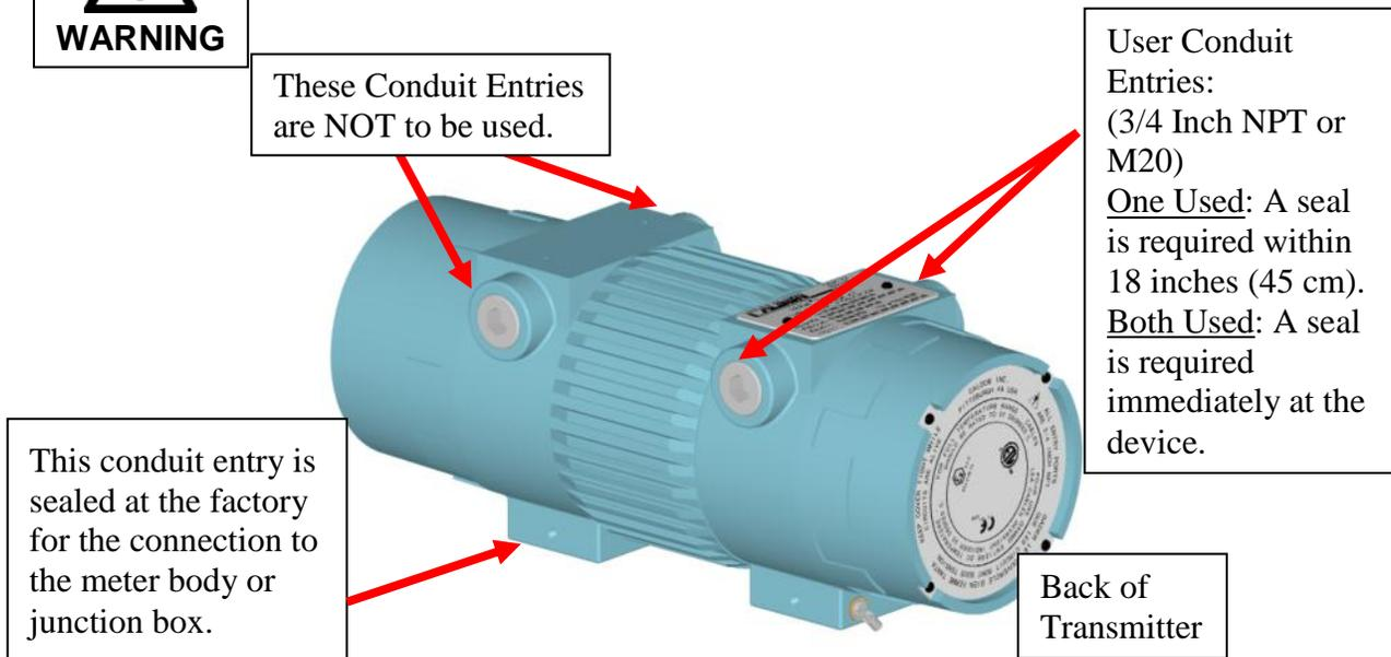
Figure 4.1: Fully Assembled Transmitter – Rear View
