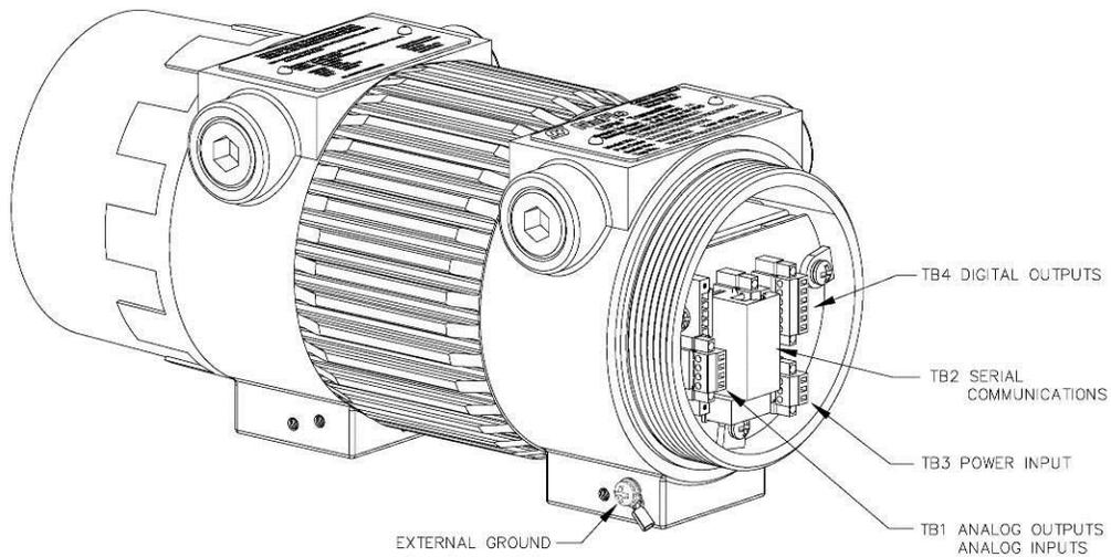
Figure 4.4: User Terminations - Cover Off (Communications Option 2)
