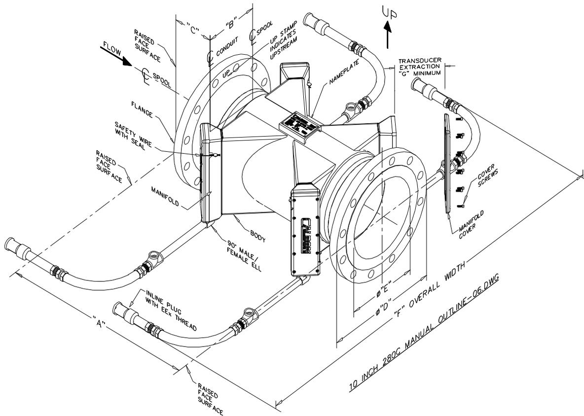
Figure 3.5: LEFM 2xxCiLT: Meter Body Termination Locations with built in connectors.
