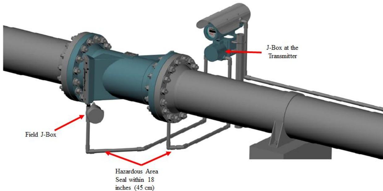
Figure 3.1: Remote Installation of Transmitter from Meter Body
