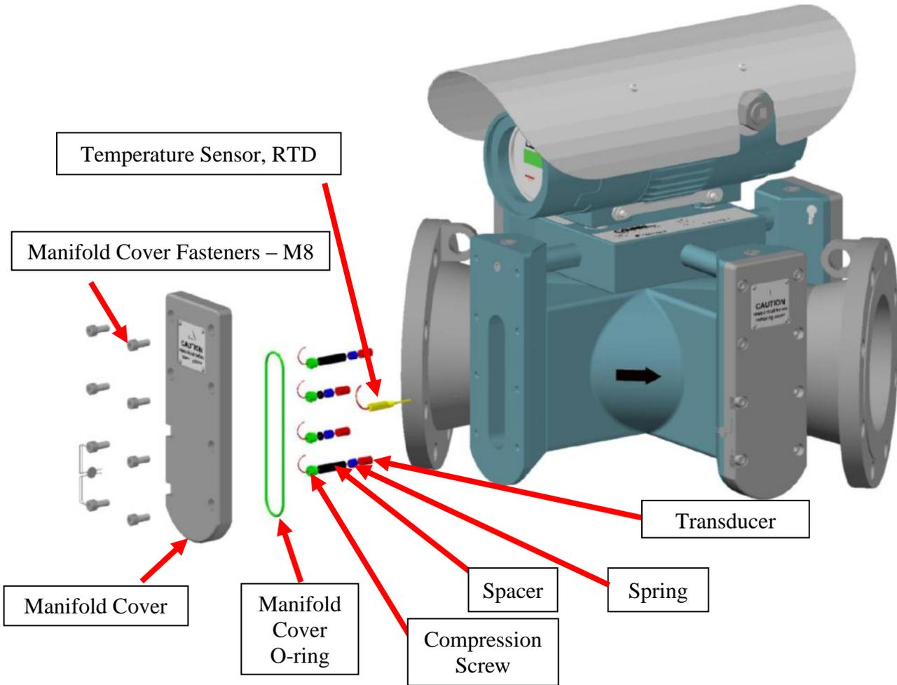
Figure 8.13: Transducer Replacement
