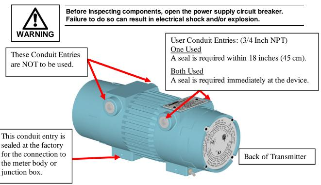
Figure 5.1: Fully Assembled Transmitter – Rear View
