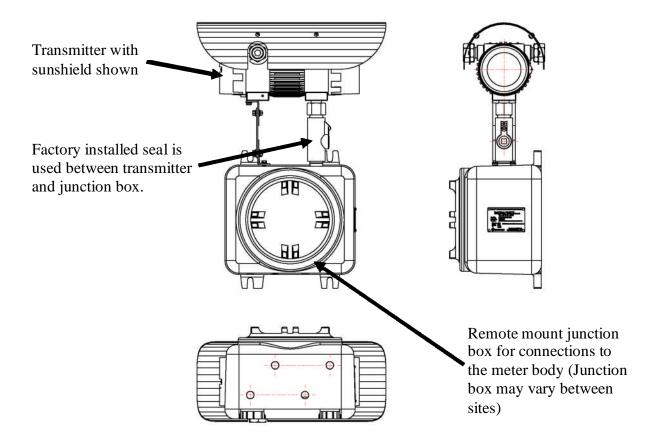
Figure 3.3: Remote Installation of Transmitter/Junction Box
