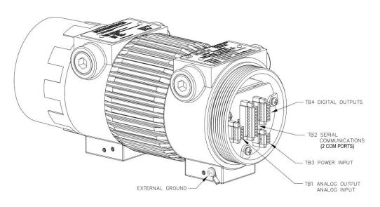
Figure 5.3: User Terminations - Cover Off (Communications Option 1)
