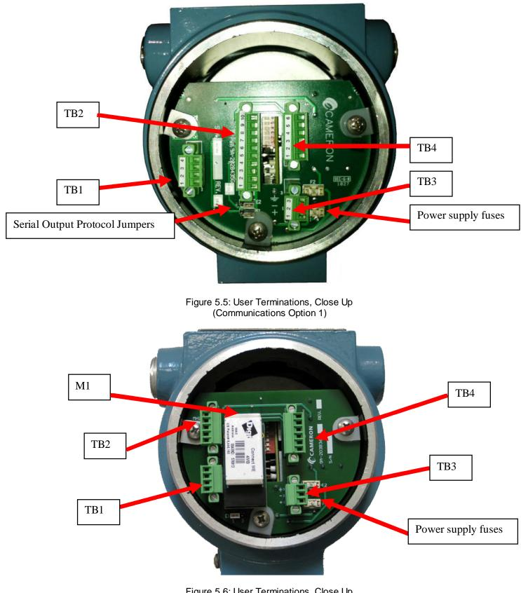
Figure 5.6: User Terminations, Close Up (Communications Option 2) Figures 5.3 through 5.6 show the location of the transmitter terminations. Inside the rear cover of the transmitter, there is a diagram of the user connections.
