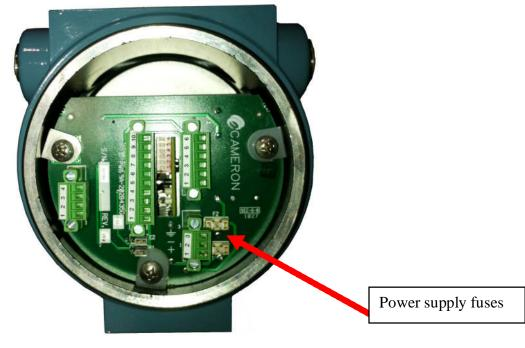
Figure 8.9: Backplane Interface Board (BIB) Fuse Location (Communications Option 1)
