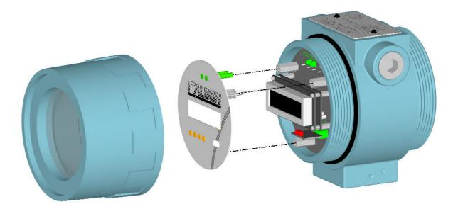
Figure 8.5: Display Cover Removal (Installation)
