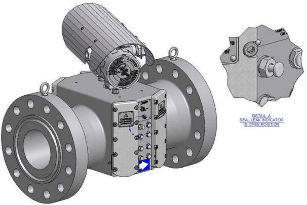
Figure 10.1: Primary Seal Failure Indication
