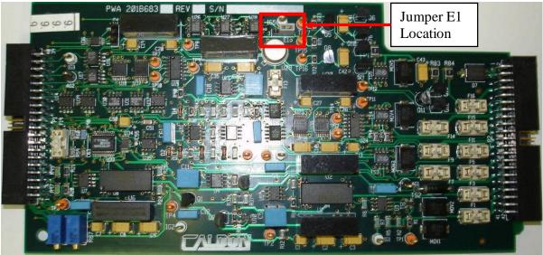
Figure 8.14: Jumper Location to Change Digital Output Voltage
