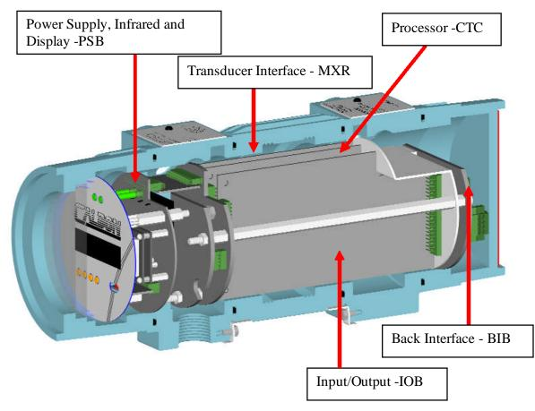
Figure 8.2: Transmitter Active Components
