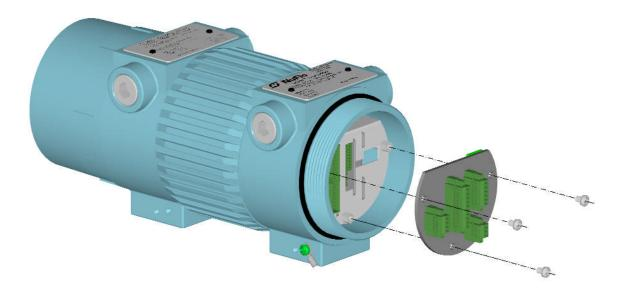
Figure 8.8: Backplane Interface Board (BIB) Removal
