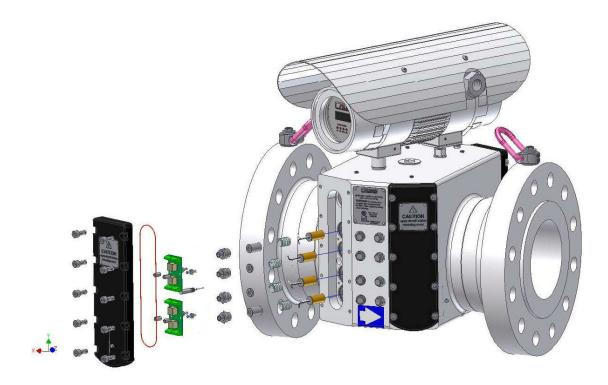
Figure 8.12: Transducer Replacement
