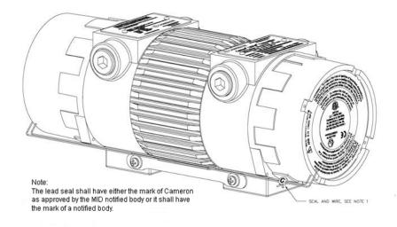
Figure 4.2: Seal Wire on Electronic Unit
