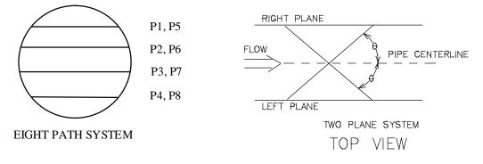
Figure 6.2: Acoustical Path Configurations
