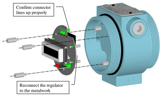
Figure 8.6: Power Supply/Display Removal/Installation
