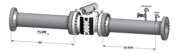
Figure 2.1: Best Practice for Installation Hydraulics
