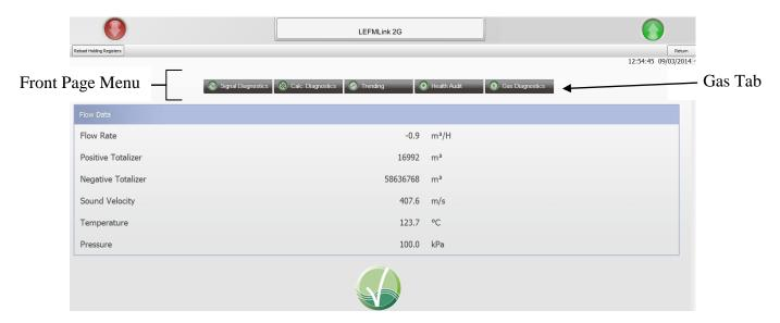
Figure 8-1 Main LEFMLink 2G screen with Gas Tab enabled
