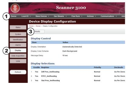
Figure 1.5—Common navigation sequence
