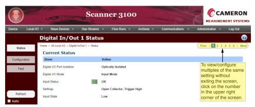
Figure 1.6—Selection options bar for configuring multiple instances of a parameter without leaving the parameter menu
