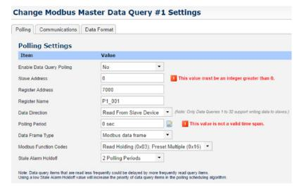
Figure 1.7—Validation errors identified with red text
