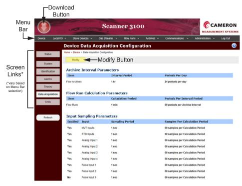
Figure 1.1—The four basic navigational features of the Scanner 3100 web interface
