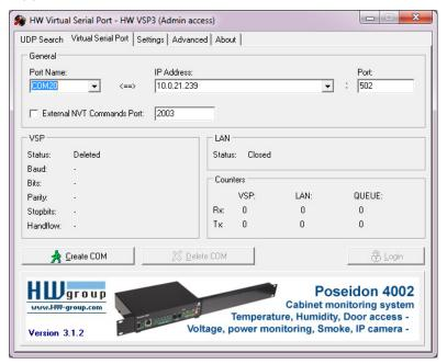
Click CREATE COM to add the virtual serial port to your computer. If the connection is successful, the VSP section of the screen will display a "Created" status, and the LAN section will display a "Connected" status.
