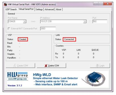
If you are having difficulty connecting through the virtual serial port, check the counters shown on the Virtual Serial Port tab above.
