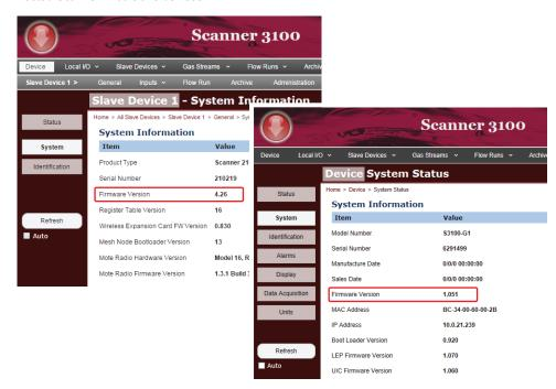
Figure 2.2—Firmware version location on Device System Status and Slave Device # System Information screens
