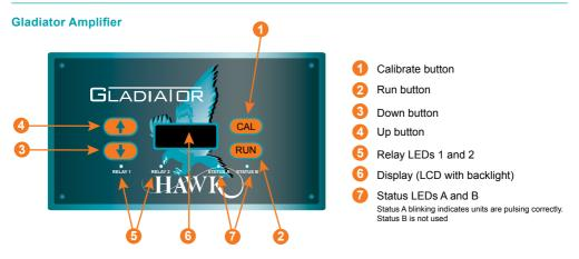
All software adjustments can be made by the push buttons on the amplifier facia.
