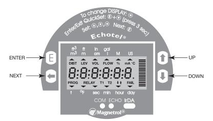
There are three LEDs in the LCD module. The ECHO LED will be continuously lit when the 335 is receiving a good signal back from a stable level surface. The ECHO LED will blink when it is receiving a signal back from a decreasing or increasing level surface. When the ECHO LED is not lit the 335 has lost the signal, and cannot make a reliable measurement. The IrDA LED is only used at the factory for software upgrades. The COM LED is not used.
