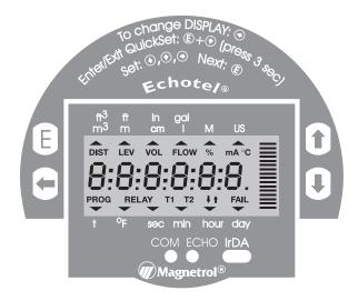
The middle row of the LCD module consists of a 6-digit alphanumeric display of all data. Engineering units for the numeric data are printed above and below the LCD. Two pointers are used to indicate which units pertain to the display that is currently being viewed. The pointer in the upper right portion of the module indicates:
