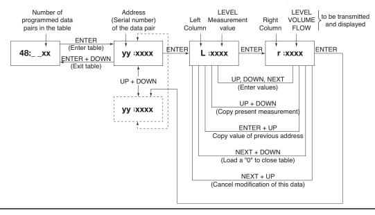
The linearization table must start off with a value being assigned to zero level in the vessel or primary flow element. This zero level is assigned to data pair point 01 as "Li 000.0" and "ri xxxx" filled in with the volume, open channel flow, or level value corresponding to the zero level value.
