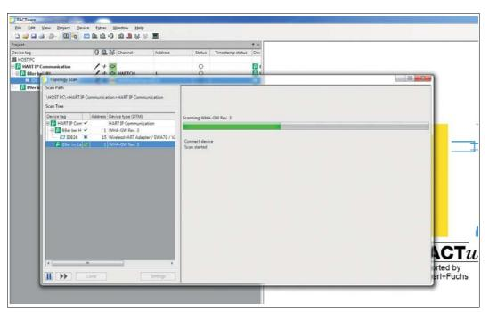
Figure 6.6 Topology scan: Filling up project tree while scanning
